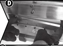
· TO INSTALL THE BLADE: hold Blade by each end and place into the Blade Slot in the Head. Be sure it is firmly seated and there is no
