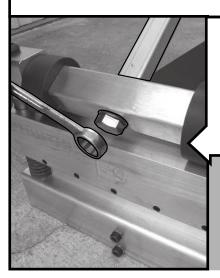
Insert M16 x 40 Bolt into Cam Shaft and tighten (24mm or 15/16" wrench recommended)
