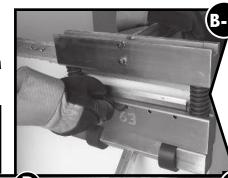
Using the 4mm Hex Wrench (included), LOOSEN BUT DO **NOT REMOVE the M8 Set Screws**. This will loosen the
