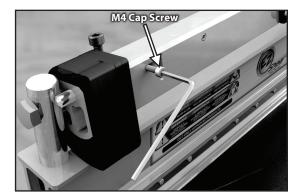
Insert the new Camlock pin and screw the M4 Cap Screw back into place. Tighten securely with the 3mm allen wrench.
