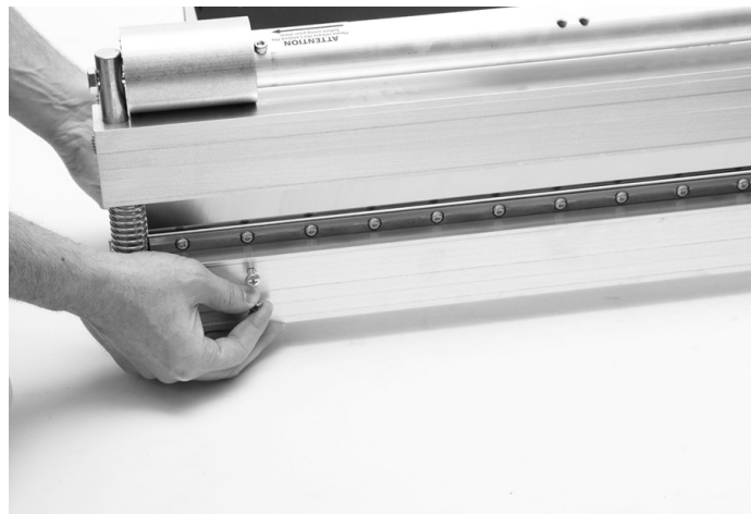
4. Attach the Shear Assembly (B) to the Bed Brace (C) using Hardware Set (H).
